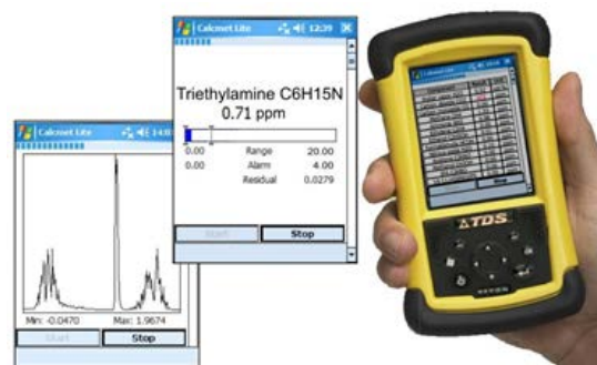
Figure 2 Calcmeter Lite and TDS Recon rugged handheld computer provide a flexible user interface. Frequently used commands have shortcut buttons while various views provide the user with detailed information
